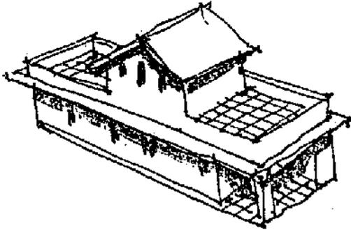
**FLAT ROOF** with an **EXTRA STOREY**. This can of course be on one part, and other part used as a terrace for drying etc. or other parts also, or over the entire ground floor plan.
