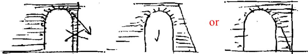
5. Frame work, templates, arch frames must be removed immediately the arch is completed (to allow for compression as the mortar dries and shrinks)
