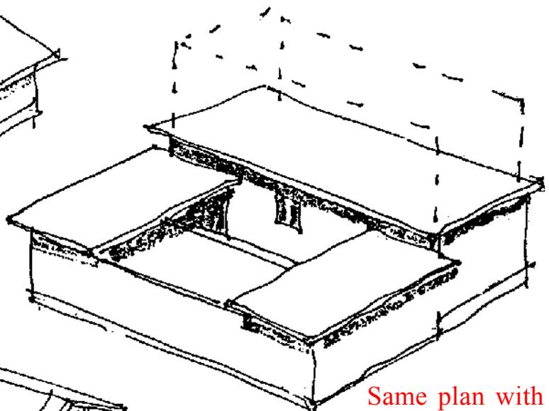
Same plan with flat roof with space for vertical expansion
