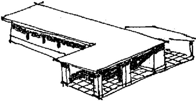
Same plan but with a longitudinal pitched roof of thatch, Tile, L pan, etc.
